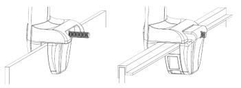
3. Choose appropriate Sliding Rail for desired front to back position \*XR15 Kit only includes two Sliding Rails.
